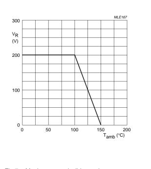
Fig.7 Maximum permissible continuous reverse voltage as a function of ambient temperature.
